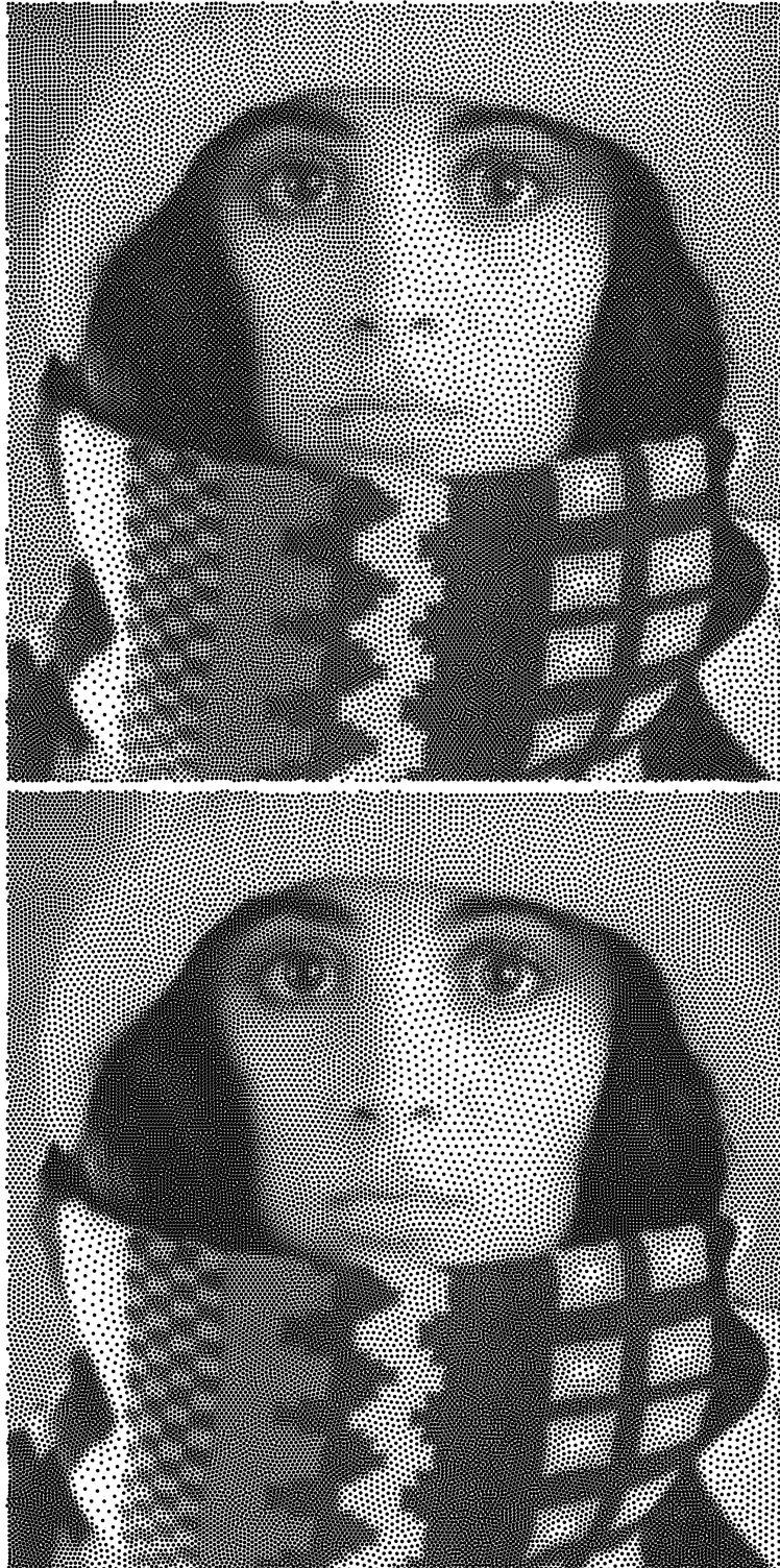
Figure 6.12: Halftoning results on the torus \mathbb{T}^2 for the left image in Figure 6.7 with M = 30150 points, which are obtained by minimizing the squared equal weights worst case quadrature error (\text{err}_{K_N})^2 , cf. (6.111), for randomly distributed initial points by the nonlinear conjugate gradient method, cf. Algorithm 3.3, for polynomial degree N = 650 after k = 744 CG iterations (top) and for polynomial degree N = 1300 after k = 21157 CG iterations (bottom). For details see Example 6.39.
