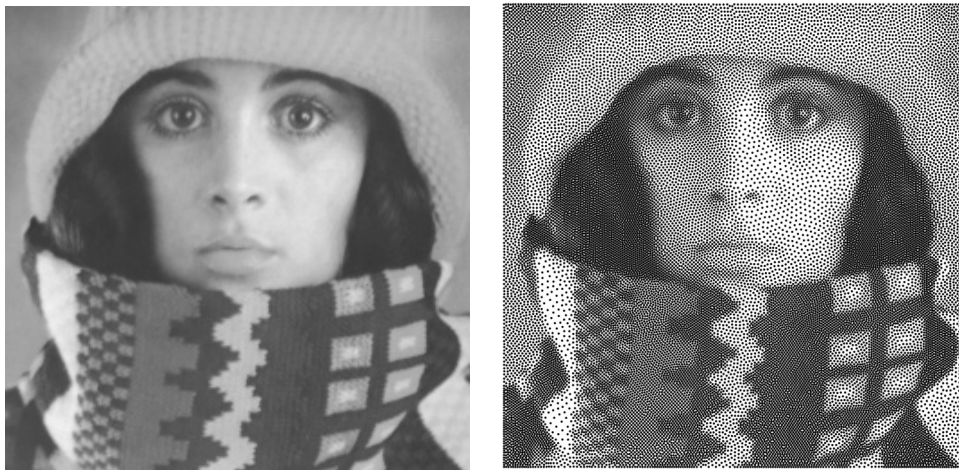
FIG. 1. Left: Original 256 \times 256 image. Right: Stippling result by minimizing (1.1) with m = 30150 points using the technique from [55].
